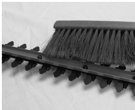
Figure 4-2: Cleaning cutter blades
